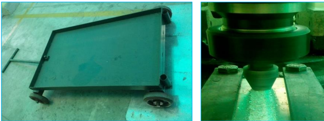
Photographs above show a Trolley, a Fixture and tool to weld aluminium plates that have been fabricated by the Participants of a training programme and M.Tech. students using the facilities of the centre.
